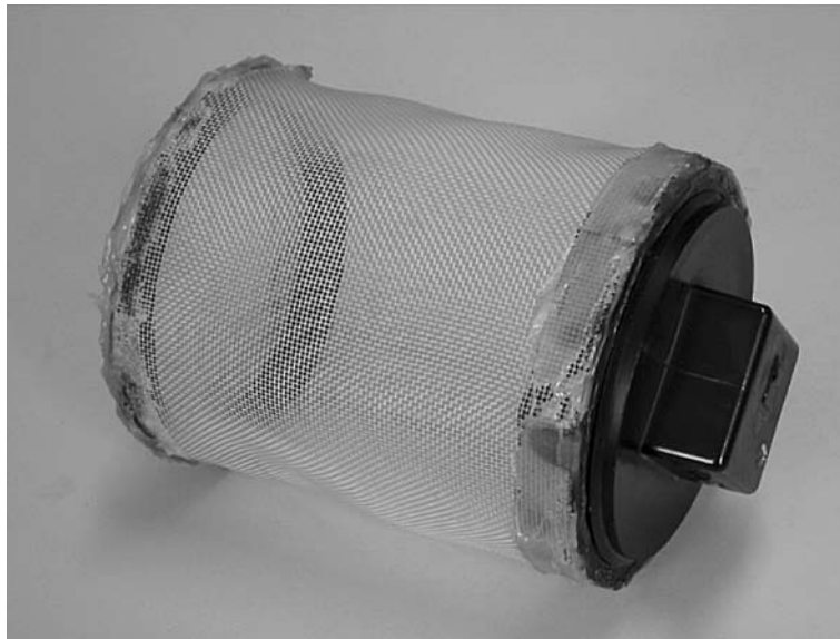
Figure 3. Photograph of one of the incubation basket used in this study. The basket has a cylindrical form (16×13 cm) and is made of 1 mm Nitex netting and ABS (Acrylonitrile butadiene styrene) plastic tubing.
